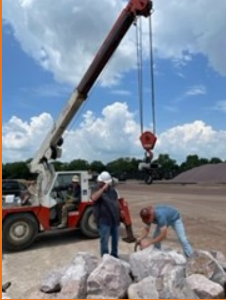
Rigging 100 lb. and larger rock for individual weights
